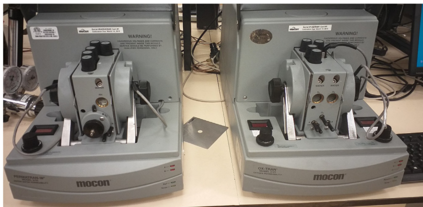
Figure 12.2 On left a Mocon Permatran-W Model 3/33 Series for measuring moisture permeability. On right an oxygen permeation rate testing device, the OX-TRAN Model 1/50.
