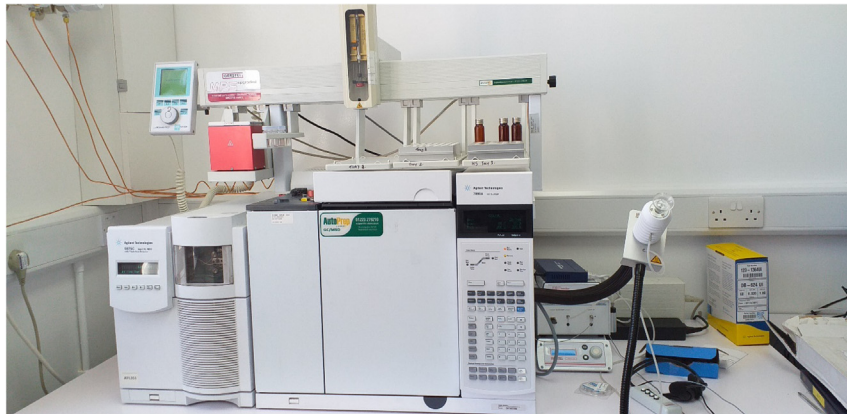
Figure 12.1 Agilent GC–MS with GCO sniffer port. GC–MS, Gas chromatography/mass spectrometry; GCO, GC-olfactometry.
