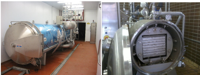
Figure 11.1 A commercial Static Steriflow Retort. The cycle used in the machine brought the temperature up to 122°C and was maintained for 5 min (to reach a 12D cycle on Bacillus stearothermophilus spores) (Left picture). Surdy Rotary Retort located at the processing facilities University College Cork (Right picture).
