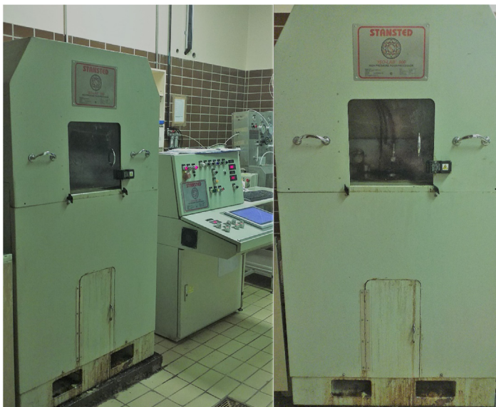
Figure 11.3 A well-used HPP rig located in the School of Food and Nutritional Sciences, University College Cork, Ireland. HPP, High-pressure processing.
