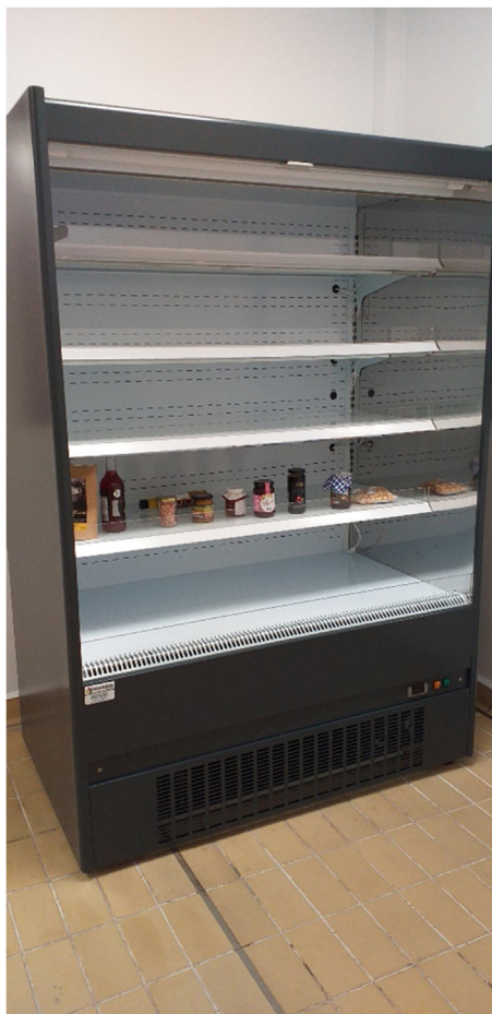
Figure 10.1 Retail display cabinet used to simulate commercial retail display conditions. It is important when using such equipment that the light intensity (LUX) is recorded as well as operating temperature fluctuations using a data logger.
