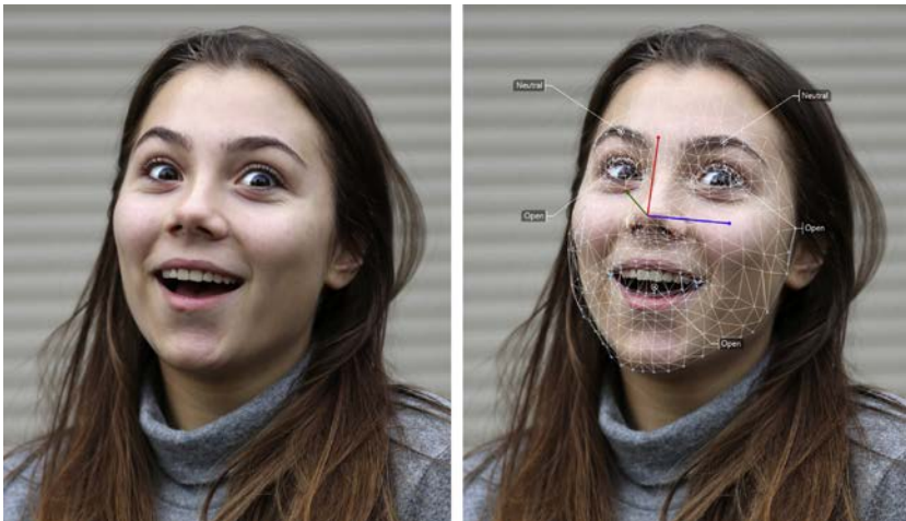
FIGURE 10.4 Example of how FaceReader software produces and visualizes the three-dimensional model of a face using 500 key points.
