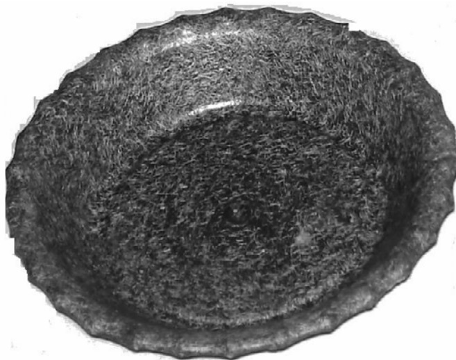
Figure 1. Extruded and injected-moulded plate fabricated with starch reinforced with fibre.
