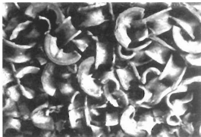
Figure 9-6D. Berl saddles (ceramic), dumped.
