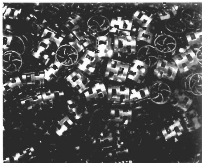
Figure 9-6E. Pall rings (metal), dumped.
