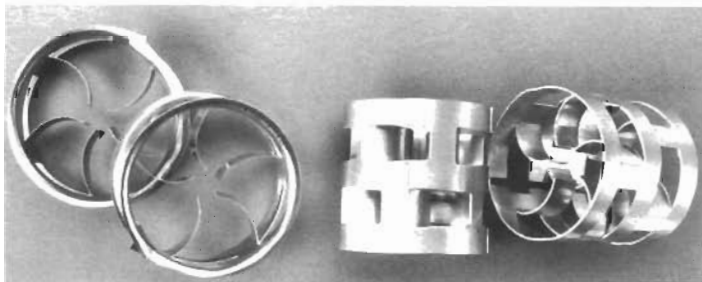
Figure 9-6T. (Top) Cascade® Mini-Ring, (metal and plastic). Originally used by permission of Mass Transfer, Inc., now, Glitsch, Inc. (middle and bottom) Elevation and plan views of Ballast® rings (right) and Cascade Mini-Rings (left). Note how high aspect ratio of former permits occlusion of interior surfaces. Low aspect ratio of Cascade Mini-Rings, on the other hand, favors orientation that exposes internal surfaces for excellent film formation, intimate mixing, and gas-liquid contact. Used by permission of Glitsch, Inc. Bull. 345.
