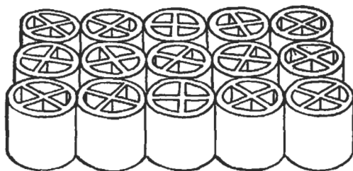
Figure 9-16A. Stacked packing: square pattern (S). Used by permission of U.S. Stoneware Co. (now, Norton Chemical Process Products Corp.).
