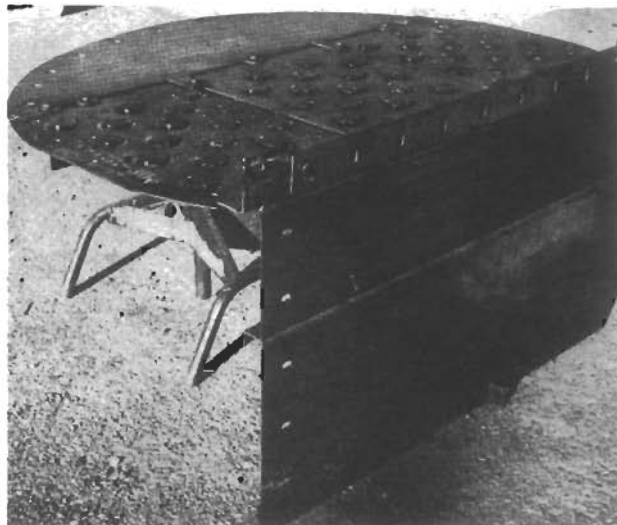
Figure 8-77. Type V-1 Ballast ® Tray. Used by permission, Glitsch, Inc.
