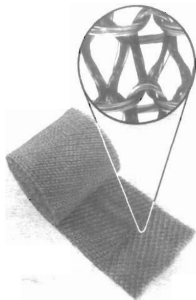
Figure 9-6CC. York-Twist™ structured tower packing. Note insert showing weave and sections fabricated to fit through manway for larger towers. Used by permission of Otto H. York Co., Inc., a division of Glitsch, Inc.
