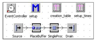
Settings: Source interval 1:30 minutes, blocking; create three entities p1,p2,p3. The source creates the parts in a cycle. Use the TableFile creation\_table for the distribution of the parts:
