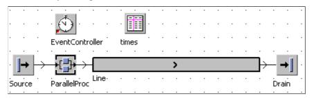
Settings: Source: interval 20 seconds, Line: length 12 meters, speed 0.08 m/s; Drain: 0 seconds processing time. To define the processing times, follow these steps:
