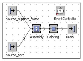
Make sure that you first connect the source\_support\_frame, then source\_part with the assembly. You have to convince the support\_source\_frame to generate support\_Frames (default is Entity). Double-click on the source and select **MU** Container.
