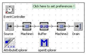
Insert a comment with the text "Click here to set preferences!" (to open the AttributeExplorer). The processing times of Machine1 and Machine2 should be changed in a single dialog box. Therefore, add an AttributeExplorer to the frame. Open the AttributeExplorer by double-clicking it. Select the tab Objects and turn off inheritance (+ Apply). Drag the items from the frame to the list of object paths. Press Enter after each object to add a new line to the table.
