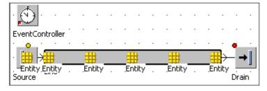
What kind of behavior the line must have depends on the technical realization of the Line. Conveyor belts or roller conveyors are normally accumulating; a chain conveyor is generally non-accumulating.
