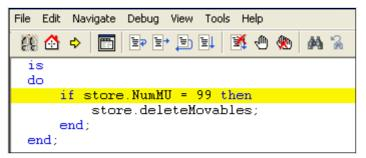
Using F11 you can, for example, move through your method stepwise and see what happens. If the method is completed, the method will open again in the editor. If an error occurs during the simulation, the debugger automatically opens and displays error messages.
