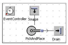
The source produces one part every minute. All other components use their basic settings. When you start the simulation, the pick and place robot transports parts from the source to the drain.
