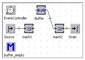
Settings: Capacity of the Buffer: 100, Source: interval 2 minutes, mach1: processing time: 2 minutes, 100% availability, mach2: processing time: 10 seconds, 50% availability, MTTR 10 minutes, mach1 exit control front: method Buffer\_empty
