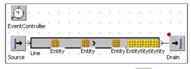
Remove the MUs from the simulation model (), then clear the checkbox **ACCUMULATING** in the dialog of the Line and confirm your changes by clicking OK. Now restart the simulation. The parts on the line keep their distance. With this setting, the line cannot be used as a buffer.
