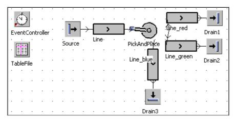
Settings: The source randomly creates part1, part2, and part3 33% each in an interval of 2 seconds. Connect the PickAndPlace object with Line\_red first, then with Line\_green, and lastly with Line\_blue. You can define the distribution of parts by color by the exit strategy of the PickAndPlace robot. Select the option **MU ATTRIBUTE** on the Tab **EXIT STRATEGY**. Then click Apply. The dialog shows additional dialog items:
