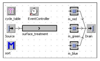
Settings: Source: interval 1 minute, sequence cyclical (cycle\_table); a cycle consists of three parts red, two green, and two blue. Create three MUs in the path models: red, green, and blue for the simulation. Color the icons according to the designations.
