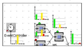
The statistical data is displayed graphically in the frame. You can also output the data after the analysis as a table. Click **RANKING TABLE** – **OPEN**. Once you have chosen a sorting option, the table is displayed.
