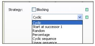
**Blocking** here means: If you select **BLOCKING**, and a transfer request could not be met, the transfer request will be entered in the blocking list of the object. It will
