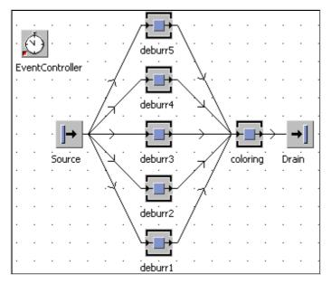
To simplify the simulation, you can use a station with five processing stations (ParallelProc).
