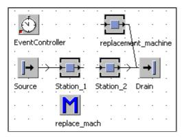
*Method replace\_mach*  $\rightarrow$  *exit control front Station\_1*
