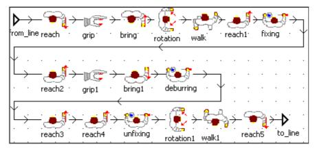
Note: In this example, you have to prevent that more than one part stays in the Frame "deburring". After an MU has entered the object "reach", the entrance of the object "reach" must be locked and may only be opened again if the part "reach5" exits. To do this, you need a method object in the Frame deburring (folder information flow). Add a method object to the Frame. Open the object by
