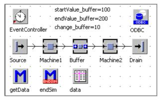
The Source produces one part (blocking) every minute. You are to save the settings and the results of the simulation into a database. Insert a database into Access and save the database under productiondatabase (.mdb). The database will initially contain two tables:
