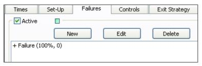
Enter the failure data into the dialog, e.g., tool change:
