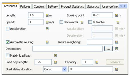
**Length**: The length of the transporter must be smaller than the length of the track, if you want to create a transporter on a track. The capacity of the tracks (setting capacity = -1) is calculated as the length of the tracks divided by the length of the transporter.
