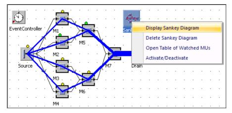
The thicker the Sankey streams between two stations, the more MUs have been transported on the connectors or methods between these stations. The exit strategy cycle of the source leads to the stations M1 to M4 receiving the same number of parts. If a machine fails, the source waits with the transfer process until the machine is operational again. M1 to M4 receive the same number of parts (Sankey lines have the same width). Output after 50 days is 21,230 parts.
