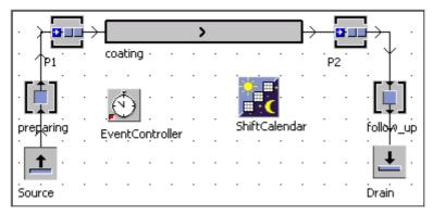
Settings: Length of the entities: 0.2 meters, P1, P2 processing time 0 seconds, capacity 10,000 parts each.
