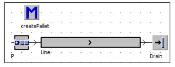
The method createPallet must first create the palette on P and then create parts on the palette until the palette is full. Create duplicates of container (Pallet, Xdimension: 25, Y-Dimension: 2) and entity (part) in the folder MUs.
