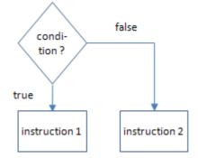
After testing a condition, the branch decides which of the following instructions should be executed. If the condition is met, the if-branch (TRUE) will be executed. If the condition is not met, the else branch (False) will be executed.
