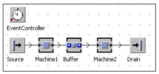
Let the simulation run for 2 days to observe the buffer. The line should not jam; the buffer should not be oversized either. You can make an evaluation of the necessary buffer size using the tab statistics of the object buffer.
