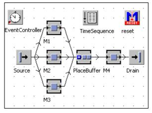
Settings: Source interval 50 seconds, blocking; M1,M2,M3 processing time 1 minute, 50% availability, 45 minutes MTTR; PlaceBuffer capacity 10,000 parts, 0 second processing time; M4 40 seconds processing time, 75% availability, 25 minutes MTTR.
