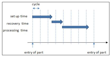
SETUP TIME: The Setup Time is the time which is required to set up a basic object for processing another type. The type is determined by the name of a MU (MUs with the same name have the same type). You can also use a setup time after a certain number of parts have been set up, for example, for regular tool changes.
