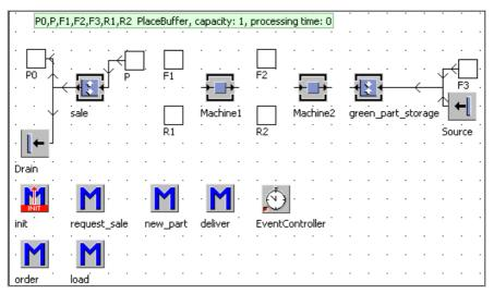
Settings: Machinel and Machine2 processing time: 1 minute, 100% availability; sale: DismantleStation, successor number 1: P0 (for containers), successor 2: Drain 1 minute processing time. Create an entity .mus.part. The source produces .mus.part, interval 1 minute. Select the following settings in the DismantleStation sale:
