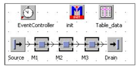
From version 9, you must create for M1, M2, and M3 first a failure. Name the failure in all three objects each "failure1". Format the table according to the following sample (take notice of the data types) and enter the data (see chapter Information flow objects – List Editor):
