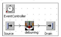
Set the interval of the source to 30 seconds. By double-clicking the object deburring you can open the sub-frame.
