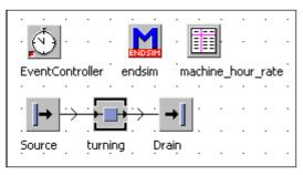
At the end of the simulation, the method EndSim reads (set a month as the end of the simulation in the event controller) the working time of the object turning from the statistics data and writes it to the table machine-hour rate (cell [1,18]). Then, the table calculates the machine-hour rate.
