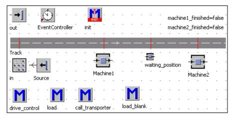
Settings: The source produces parts at an interval of 3:30 minutes. The processing time of Machinel is 7:50 minutes, of Machine2 7:40 minutes. Both machines have an availability of 90% and an MTTR of 45 minutes. The track has a length of 25 meters; the transporter has a length of 1.5 meters, a speed of 1 m/s and a capacity of one part. The capacity of the object in is one part. Insert the following sensors into the track (as the drive control):
