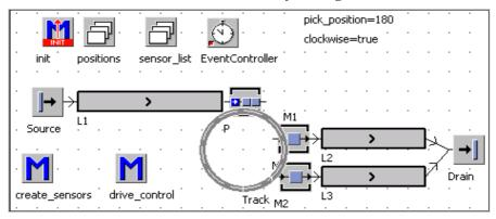
Settings: Source interval 30 seconds, Buffer P processing time: 0 seconds, capacity one part; M1 and M2 each 55 seconds processing time; L1, L2, and L3 each 1 m/s speed.
