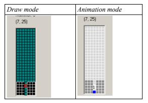
The reference point is located at the lower end of the icon. There also is an animation point for the MU which is to be transported. The orientation and size must be coordinated with the robot.
