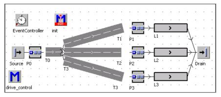
Length of the tracks T0: 0.2 m, W1: 0.75 m, W2: 0.7 m, W3: 0.75 m, processing time P1, P2, P3 3 seconds (to secure a distance between the parts), the capacity of all buffers is one part. The length of the transporter is 0.1 meter (booking point 0). The transporter must drive backwards after being inserted into the frame. Therefore, select Backwards in the dialog of the transporter in the class library. Proceed as follows.
