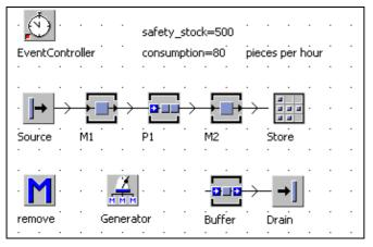
Settings: Source interval 1 minute blocking, M1 and M2 processing time 50 seconds, availability 95%, MTTR 5 hours, P1 capacity 1000 parts, store capacity 10,000 parts. Create safety\_stock and outward stock movement (consumption) as global variables, of data type integer, in the frame
