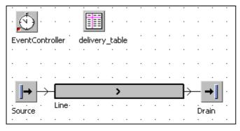
Duplicate the object Entity three times in the class library. Rename these duplicates to part1, part2, and part3. The source should produce five parts of type part1 after 2 minutes, two parts of type part2 after 10 minutes, and four parts of type part3 after 15 minutes. Select **TIME OF CREATION – DELIVERY TABLE** in the dialog of the source. Next, click in the lower part of the window on the button with the three points. Select the table in the following dialog.
