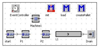
Settings: Start, P1, P2 each one place, processing time 0 seconds, L1 4 meters length, speed 1 m/s, Machine1 processing time one minute, no failures.
