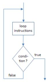
The condition is checked after the execution of the loop statement. If the condition for a termination of the loop is not met, the loop statement will be executed one more time. The loop statement is executed at least once.
