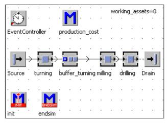
Material costs of unfinished part:  $\epsilon$ 24.95, average manufacturing wage  $\epsilon$ /h36. First, the part is turned, then milled, and then drilled. Processing times: turning 1 minute, milling, drilling 1 minute. The relevant entity (Part) is to have the property "production\_cost" (data type real).
