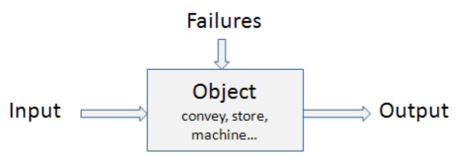
The individual objects and the operations within the objects are linked to an overall process. This creates a Frame. With the objects and the Frame various logistical systems can be modeled.
