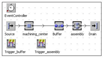
Settings: Source 1 minute interval, blocking; machining\_center 1 minute processing time; buffer 0 second processing time, capacity 1000 parts.
