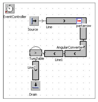
Enter the following settings: The source generates the MU partarrow at intervals of 1 minute. Leave the basic settings for all other objects. Start the simulation and track the movements of the part.
