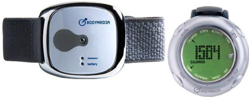
Fig. (5). Wireless transmitter and receiver of the Sensewear multi-functional device.
