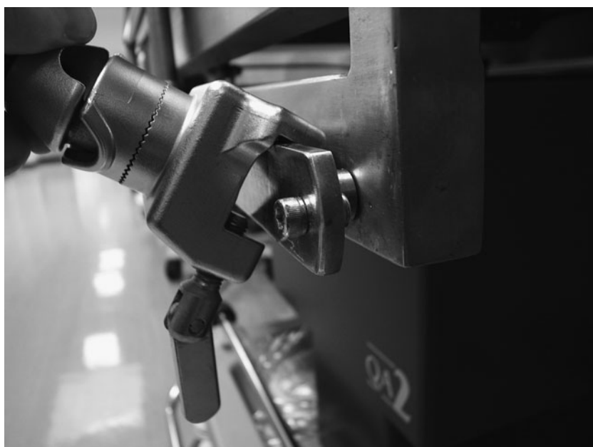
Fig. 2.10 Even though the leg supports had supposedly been secured to the operating table, when the surgeon checked it proved possible, with minimal force, to detach the leg support. These particular leg supports had not been specifically designed for the particular type of operating table - but there was nothing to prevent their use on the wrong table! Always check yourself that the leg is secure.
