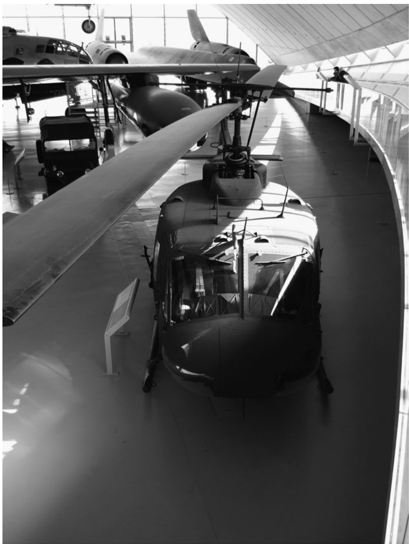
Fig. 7.4 The rotor of this Huey helicopter is held in place by a single bolt. If this bolt fails, the helicopter will crash, hence the nickname of 'Jesus bolt' given to the bolt by US aircrew who flew these helicopters during the Vietnam war (©Oxford Urology Courses, Permission granted).
