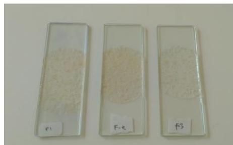
Gambar 4 Uji Homogenitas Gel
