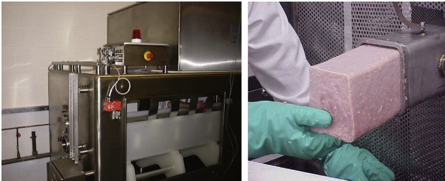
Figure 8.30 Continuous cooking of pumped meats with RF. Courtesy of Petrie Technologies.
