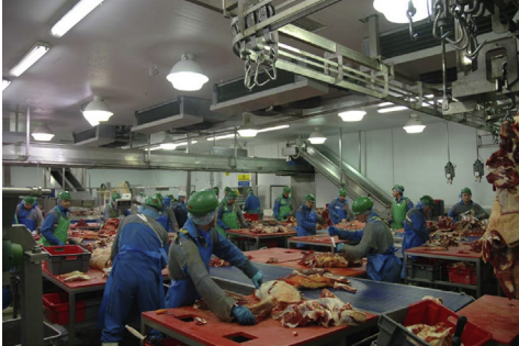
Figure 4.48 (a) Uncluttered ceiling with lighting having a sloped body with the lower part provided with a polycarbonate glass ( Courtesy of Veelite Technologies, Ltd. ). (b) Uncluttered ceiling. Lighting can be built in into the false ceiling with a hermetically closed seal and further separated with a transparent polycarbonate glass from the process area just below. It is a procedure typically for high hygiene areas where lamps are changed via the technical area ( Courtesy of Environmental Systems Corporation, ESC Cleanrooms (Moerman, 2011b) ).
