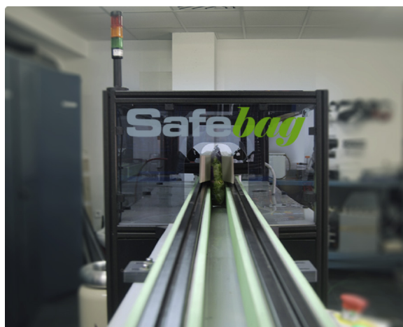
Figure 9.5 Industrial continuous plasma prototype for decontamination of fresh produce.
