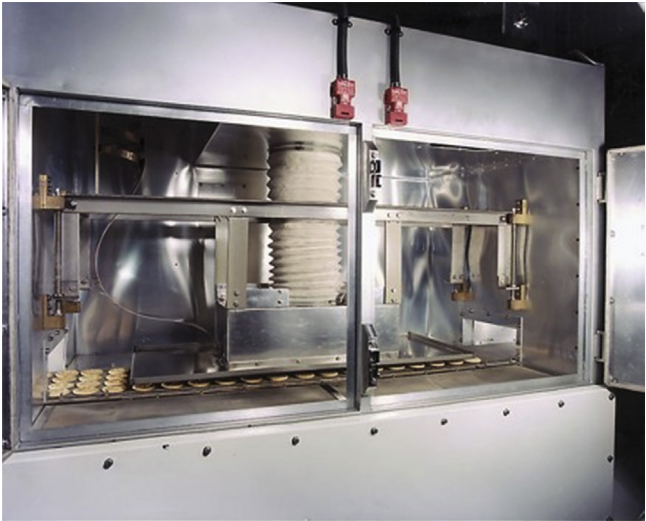
Figure 8.24 ARFA baking applicator. Courtesy of Petrie Technologies.
