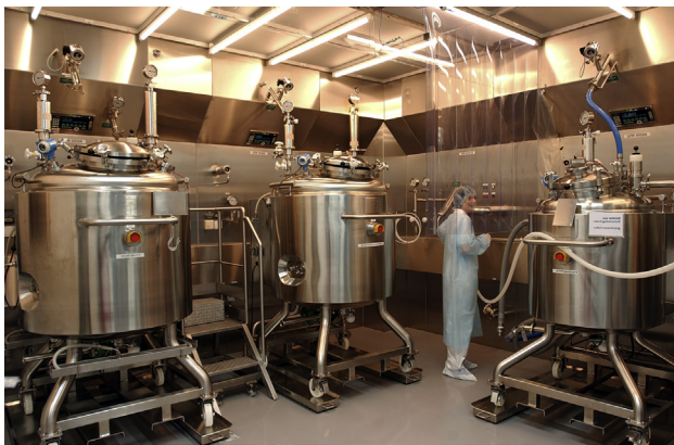
Figure 3.3 Decoupling the operating process from the facility is common sense in the biopharmaceutical industry, where wheeled and skid mounted process units are moved in and out. With this way of working, the production area can be easily modified for other manufacturing purposes.
