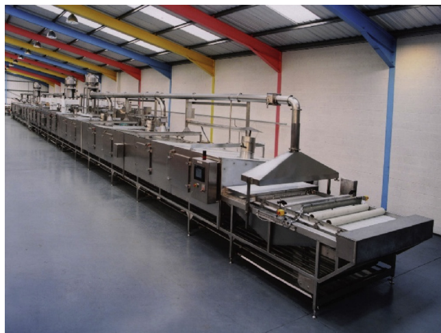
Figure 8.27 Industrial microwave/steam cooking process. Courtesy of Petrie Technologies.
