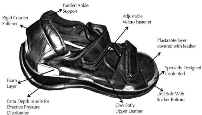
FIGURE 8 The newly developed footwear and its details.
