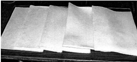
FIGURE 2 Photographs of developed PU sheets with various concentrations.
