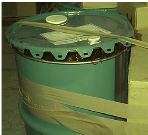
FIGURE 8.9 A clearly damaged grease container on arrival in the factory site. This grease should not be used because it will no longer meet the requirements of a food-safe product (Steenaaard et al., 2009).
