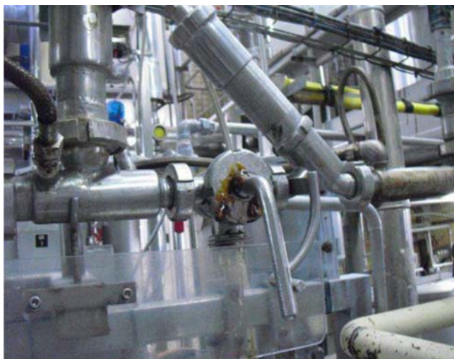
FIGURE 7.64 With respect to plug cock valves, product can get caught as a thin stagnant film around the clearance between the plug and the valve body during rotation of the plug, and finally may leak to the outside. Courtesy of Mondelez International, © 2016.
