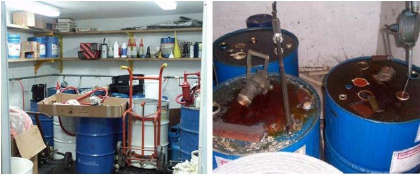
FIGURE 8.38 Incorrect storage: contamination and use of incorrect lubricants can easily occur (Steenard et al., 2009).
