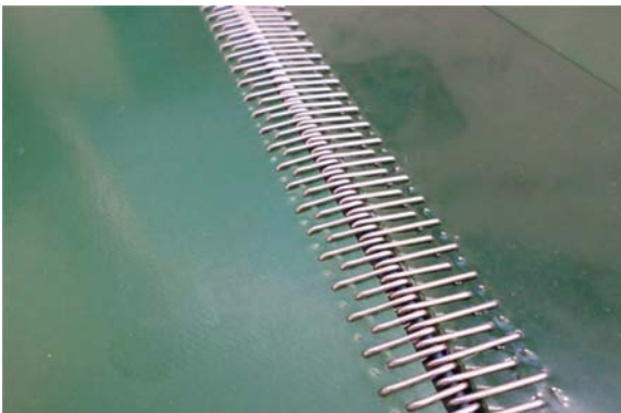
FIGURE 8.30 Wire hooks to make conveyor belts endless are not hygienic. Due to the perforation of the conveyor belt, the reinforcing fabric layer becomes exposed, allowing liquids to penetrate into the interior of the conveyor belt by wicking (capillary action) (Kold et al., 2016).
