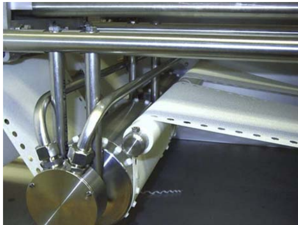
FIGURE 6.71 Cables can be protected from dirt layering and damage by encapsulating them in hermetically closed cable housings such as stainless steel pipes, especially in the neighborhood of the food contact and splash area ( Den Rustfri Stålindustri's Kompetencecenter, 2006 ).
