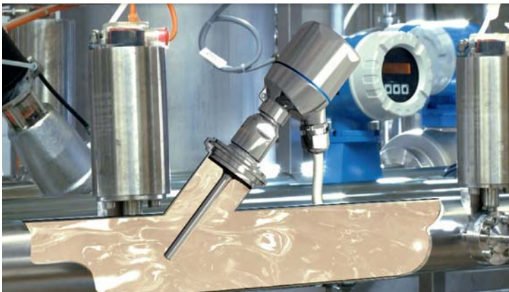
FIGURE 7.93 Temperature measurement device mounted on a upwards sloped tee branch. The length of the up-stand is not larger than its diameter ( l \leq d ). Sloped mounting of the instrument branch decreases the risk of reduced turbulent flow conditions in the instrument branch during cleaning operations. As turbulence in the sloped instrument branch is higher, stagnation of air in the upwards sloped tee is also less likely to occur. Courtesy of Endress + Hauser AG.
