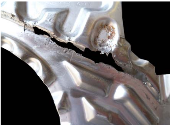
FIGURE 8.5 Plates in a plate heat exchanger may crack by overtightening or when the plate heat exchanger is opened or closed in the wrong way. Courtesy of Thermo Logistics Ltd.
