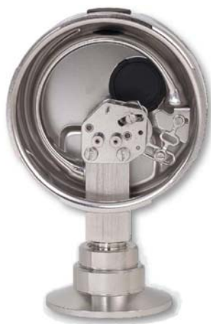
FIGURE 7.88 Mechanical gauges in particular, such as the bourdon gauge, require a diaphragm seal. Diaphragm seal gauges can cope with a greater range of process temperatures and aggressive products. Courtesy of WIKA Alexander Wiegand SE & Co. KG.
