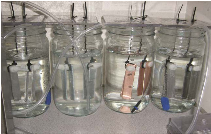
FIGURE 8.10 The compatibility of several materials of construction with detergent and disinfectant solutions can be tested in the laboratory by means of immersion tests conducted with coupons. Courtesy of Evapco Inc. Moerman & Fikiin, 2015.
