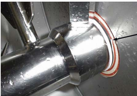
FIGURE 6.17 Stirrers, homogenizers, or mixers installed via a side wall require sealing of the shaft at the product side. When the seal is worn, however, leakage of product to the outside and product contamination may occur. Particles of the broken seal act as foreign body contaminants, and the food may be spoiled with microorganisms migrating out of the gap in which they could grow due to the presence of nutrients. www.ourfood.com , courtesy of Karl Heinz Wilm, © 2016.
