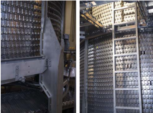
FIGURE 6.20 A metal sheet frame and subframe ending in metal sheet legs may provide higher strength than hollow framework members. The open profile framework members of this spiral freezer are still perfectly cleanable as they are turned outward. Courtesy of JBT FoodTech, a Frigoscandia freezer.
