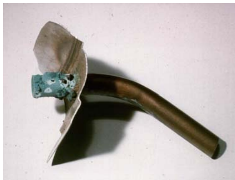
FIGURE 7.1 A badly corroded copper pipe is entering a large stainless steel hot water tank. Stainless steel is cathodic to copper in fresh water. Where the area ratio of stainless steel to copper is large, severe galvanic corrosion can occur.
