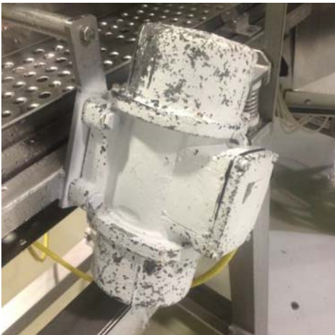
FIGURE 8.12 This motor is constructed from mild steel, and is used to impart vibration to a perforated stainless-steel bed laden with food products. During hose-down operations, the cleaning agents and high pressure typical for traditional manual cleaning procedures have ruptured the physical integrity of the paint and allowed peeled-off paint to splash onto the cleaned conveyor bed. As a result, food products subsequently produced on this process line may become contaminated. Courtesy of Joe Stout, Commercial Food Sanitation LLC - Intralox, © 2016.
