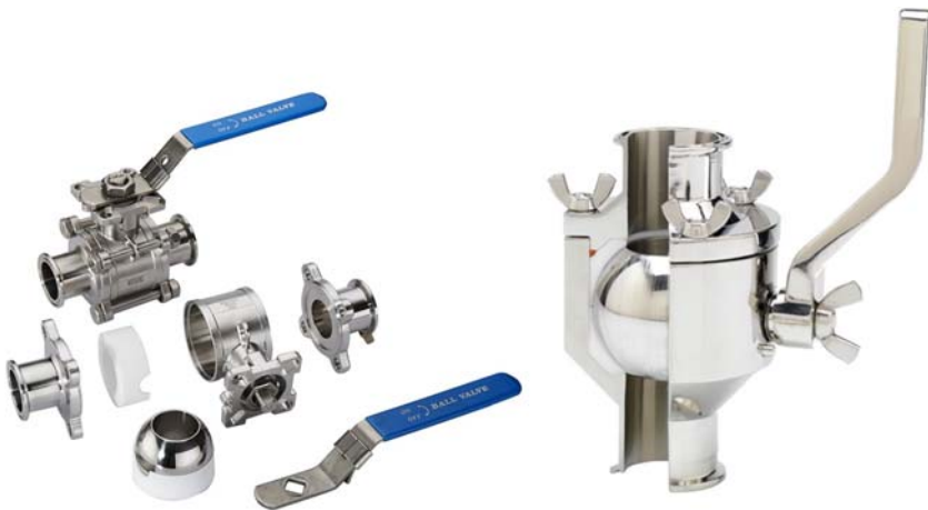
FIGURE 7.56 Cavity filled ball valves have special seat design that fills the gap (dead space) around the ball. Surfaces of the ball and valve body in contact with the product have a smooth finish with R_a < 0.8 \mu\text{m} . The ball valves are easy to dismantle allowing for inspection, cleaning, and maintenance. Photo left, courtesy of Kaysuns Industry Ltd.; photo right, courtesy of Lee industries Inc.
