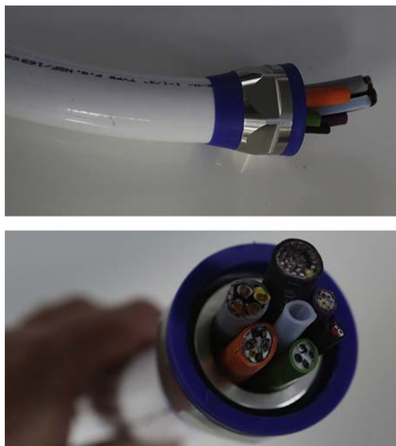
FIGURE 6.72 Multiple cables and wires can be combined in a flexible conduit with a smooth outer surface, further provided with a hygienic connector allowing a watertight connection to the maintenance enclosure or process equipment without visible thread in the screwed state. These hygienically designed conduits may reduce the number of cables that must be individually laid on cable ways, reducing the amount of contaminants that may build up on current carriers and enhancing the cleanability of the cable transport system. These flexible conduits are also suitable for connections to machinery subject to vibration (e.g., motors) (Moerman & Wouters, 2015). Courtesy Anamet Europe B.V.
