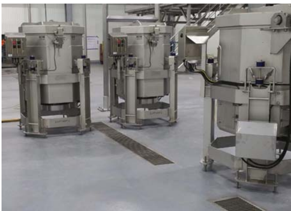
FIGURE 6.21 Channelized frame construction eliminating hollow tubes and threaded leg adjusters. Courtesy of Rudi Groppe, Heizen Manufacturing International, © 2016.
