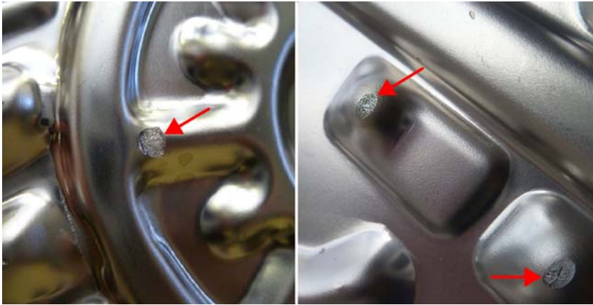
FIGURE 8.6 Plates in plate heat exchangers may suffer from surface damage, usually caused by a hard foreign body getting into the heat exchanger. The damaged spots show increased surface roughness which may promote the adhesion of food constituents (e.g., proteins in milk) and biofilm formation. Courtesy of Thermo Logistics Ltd.
