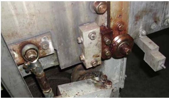
FIGURE 6.10 The process equipment is overlubricated with a nonfood-grade red grease. Courtesy of John Butts, Land O'Frost, © 2016.
