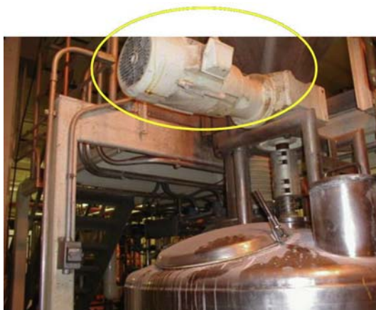
FIGURE 6.53 Drive motor is installed above the manhole of the process vessel. When the manhole cover is open, the product may become contaminated with lubricants, condensate, or dirt discharged from the drive motor ( organization Sanitary Design Workshop , © 2016).
