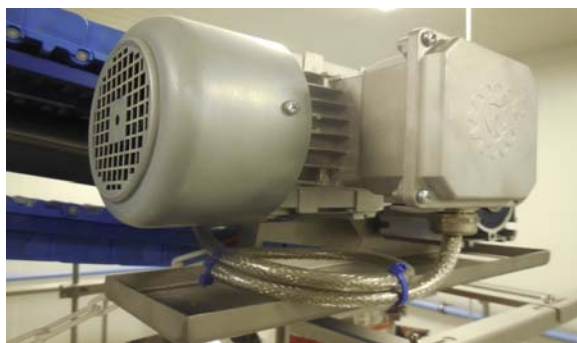
FIGURE 6.46 Although the drive motor has a drip pan, the difficult-to-clean motor is located too close to the product flow, because the fan may blow dust and dustborne microbes around and onto the food. Frank Moerman, © 2016.
