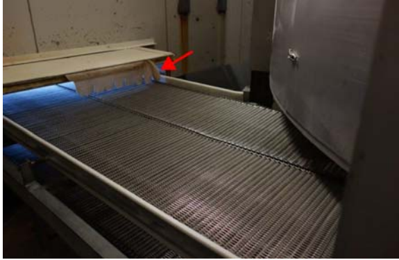
FIGURE 8.3 Ripped-off pieces of a plastic strip curtain have been lost as foreign body contaminants in the product stream, while the remaining plastic strips are extremely dirty. The plastic strip curtain is also no longer suitable to reduce the infiltration of warm humid air, and has become a serious source of microbial cross-contamination, especially for exposed products (Moerman and Fikiin, 2016). (Frank Moerman, © 2016).
