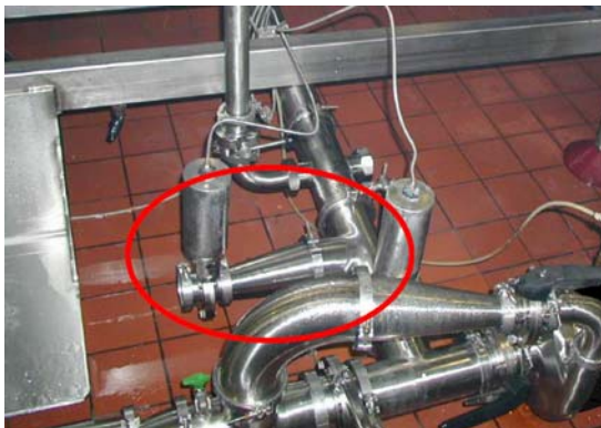
FIGURE 7.4 The too-long T-piece functions as a dead leg, where fluid movement is reduced. Courtesy of Mondelez International, ©2016.
