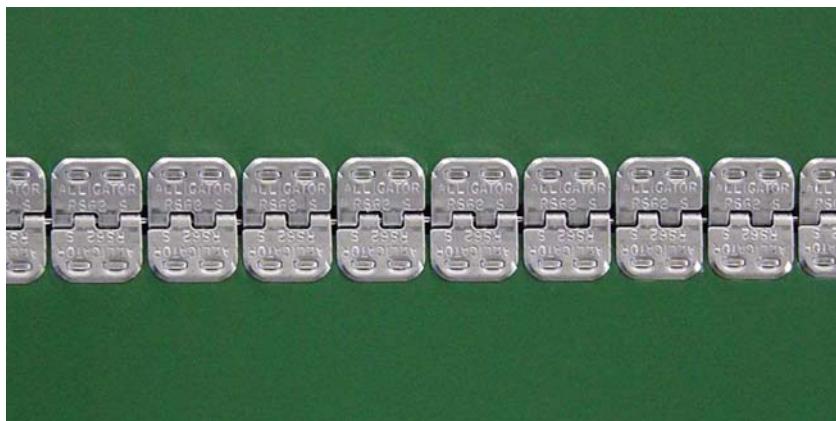
FIGURE 8.31 Staples to joint belt ends together are not hygienic (Kold et al., 2016).
