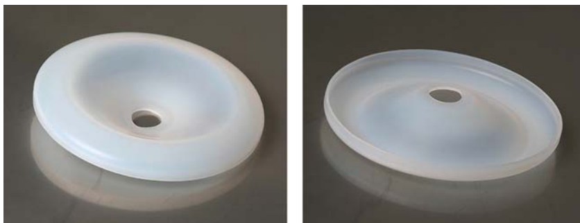
FIGURE 7.59 Diaphragm made from uniform and flexible PTFE with improved cold flow performance, and suitable for a high number of load changes. The risk of pocket or crack formation, typical for multicomponent systems, is absent (Ladenburger, 2015). Courtesy of Pentair Südmö GmbH.
