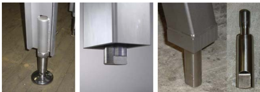
FIGURE 6.34 Adjustable feet with the threaded spindle completely concealed in closed profiles/pipes. In the first example (photo on the left), the thread of the foot is covered by the closed pipe, welded in a sheet metal leg ( courtesy of Den Rustfri Stålindustri's Kompetencecenter ). In the second example (photo in the middle), the foot can be screwed in and out at the bottom of the frame's legs ( courtesy of Alfa-Laval AB ), while the thread still remains covered in the leg. In the third example (photo right), the leveling foot is screwed in leveling foot mount ( courtesy of Schenck Process LLC ). In the second and third examples, the contact surface of the feet with the floor is rather small, which will locally exert a (very) high pressure, especially if used to support heavy equipment prone to vibration/oscillatory movement.
