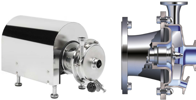
FIGURE 7.42 A casing with drain valve at the lowest point of the centrifugal chamber can be used. This solution where the pump's outlet is pointing vertically upwards while being self-draining prohibits the accumulation of air in the upper part of the casing. The drain pipe section of the drain valve must be as short as possible, because otherwise the drain valve becomes a dead leg on its own. The front cover can be removed to allow cleaning of the impeller area. Courtesy of Packo.
