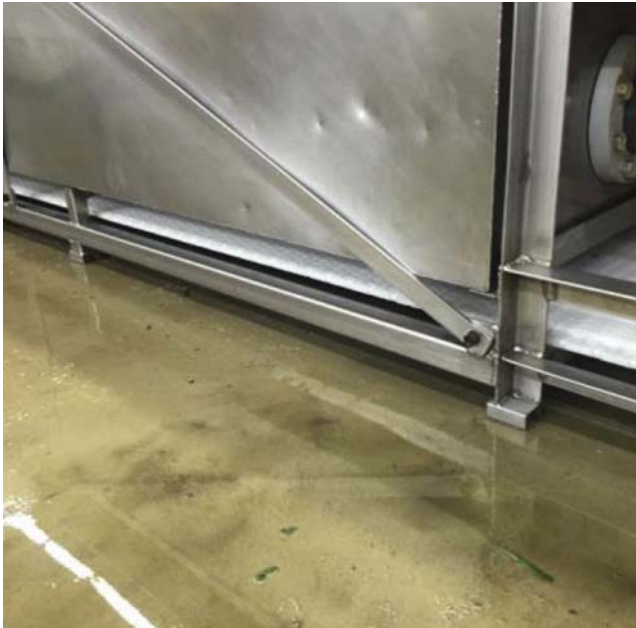
FIGURE 6.79 Process equipment should be installed as high off the ground as possible to facilitate cleaning and reduce the risk of cross-contamination during cleaning operations. In this case, dirt released from the floor during high-pressure cleaning may splash on the process equipment. Courtesy of Joe Stout, Commercial Food Sanitation LLC - Intralox, © 2016.
