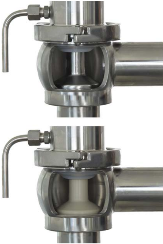
FIGURE 7.60 Linear plug and stem valves where a PTFE diaphragm with superior mechanical characteristics provides hermetic protection of the spindle travel during aseptic applications. Contrary to bellow sealed linear plug and stem valves, this valve is suitable for process operations handling liquid food with abrasive particles or products that crystallize in the atmosphere, such as lactose or instant coffee. Courtesy of Pentair Südmö GmbH.
