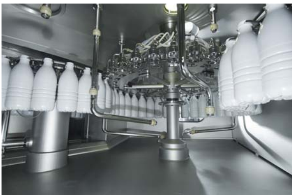
FIGURE 6.7 Equipment surfaces in the product zone must be self-draining, and internal angles and corners well radiused. Courtesy of Krones AG.
