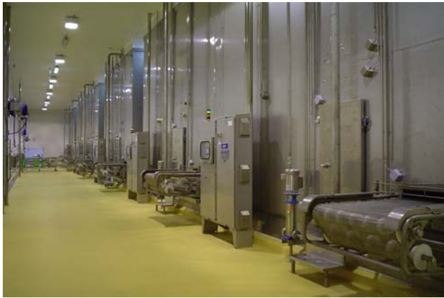
FIGURE 6.63 Sufficient distance is maintained between the cabinet base and the floor. The cabinet is positioned at a considerable distance from the wall of the enclosure. The top roof is sloped toward the front. The field boxes in smooth plastic are mounted at 45 degrees and sealed to the wall of the enclosure. Connections of cables and wires to field boxes are sealed. Courtesy of GEA Group.
