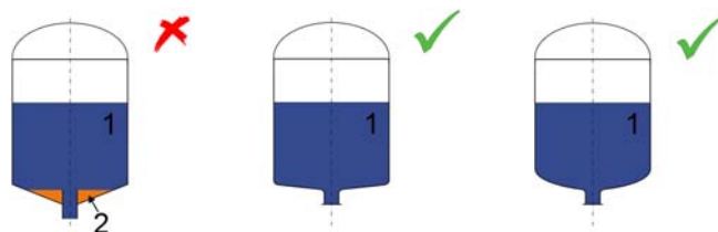
FIGURE 7.5 Full drainage of products and cleaning solutions is required. If discharge outlets are above the lowest level of the closed vessel, self-draining will be hampered, and residual products and cleaning solutions (2) will be left in the vessel. Closed vessels must be self-draining with discharge outlets at the lowest level. Bottoms must be sloped and all corners should be well-rounded (Hauser et al., 2004b).
