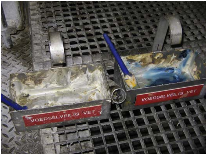
FIGURE 8.37 The blue colored brushes used for applying the lubricant are not suitable. They have turned the lubricant from white into blue. Furthermore, the lubricant stored in the “in-use” container has been cross-contaminated with other non – food-grade lubricants, and has been exposed to the environment for too long, which has allowed dirt, pests, water, microorganisms, etc., to contaminate the lubricant. The container has also not been cleaned for a long time (Steenard et al., 2009). Courtesy of Van Meeuwen Lubrication B.V.
