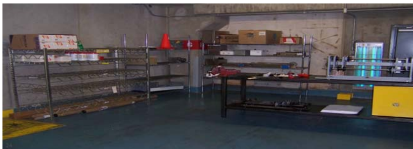
FIGURE 8.49 Storage room for replacement parts, maintenance tools and maintenance aids should be neat and clean, and allow storage in dry conditions. Courtesy of Mondeľz International, © 2016.
