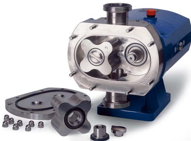
FIGURE 7.46 Nowadays there are hygienically well-designed rotary lobe pumps available with the ports arranged in the vertical plane. Slots in the rotor retaining nuts create turbulences in the flow passing the narrow gap between end cover and lobes. They provide enhanced cleanliness of the end cover and the front surfaces of the lobes. Courtesy of Alfa Laval AB.
