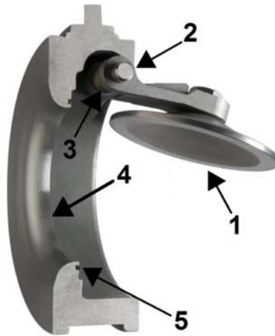
FIGURE 7.67 This nonreturn valve of the swing type consists of a disc (1) which opens in the right direction of flow by means of a hinge (2). When the flow goes in the reverse and wrong direction, the spring (3) forces the disc toward the seat (4). As an O-ring is contained in the groove of the body's seat, a uniform zero leakage seal is obtained. This design contains plenty of dead areas, and the hinge and spring are sensitive to contamination. Also the valve's drainability can be questioned.
