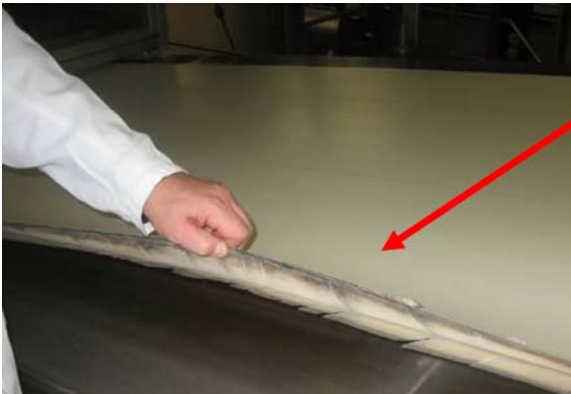
FIGURE 8.2 Damage at the edge of a conveyor belt. www.ourfood.com , courtesy of Karl Heinz Wilm, © 2016.
