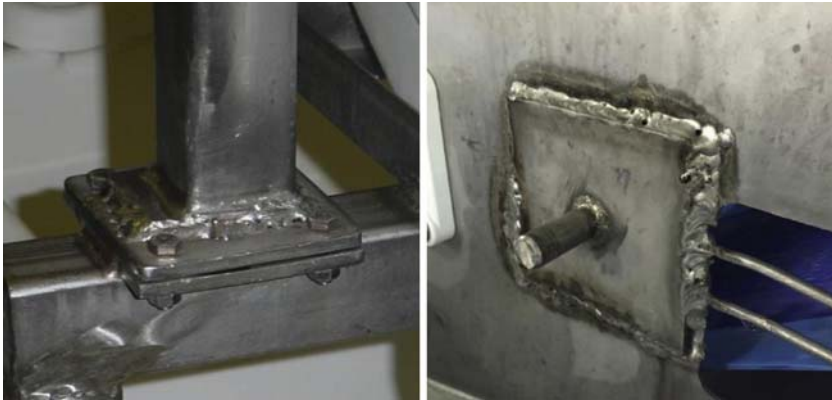
FIGURE 6.3 Welds must be continuous and smooth, free of pits and cracks. Gaps, lap seams, bolts, and threads will accumulate dirt and will make this equipment not cleanable. Photo left, courtesy of John Butts, Land O’Frost, © 2016; photo right, courtesy of Joe Stout, Commercial Food Sanitation LLC - Intralox, ©2016.
