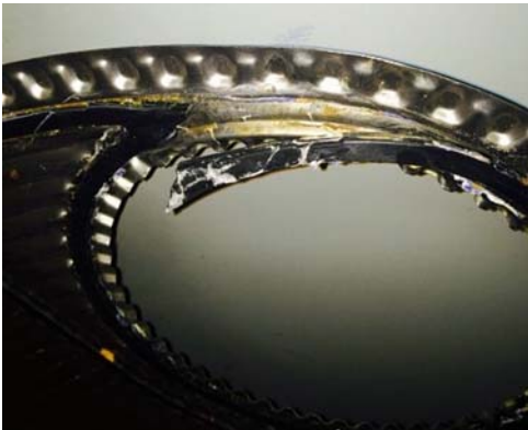
FIGURE 8.3 Ripped-off pieces of a plastic strip curtain have been lost as foreign body contaminants in the product stream, while the remaining plastic strips are extremely dirty. The plastic strip curtain is also no longer suitable to reduce the infiltration of warm humid air, and has become a serious source of microbial cross-contamination, especially for exposed products (Moerman and Fikiin, 2016). (Frank Moerman, © 2016).
