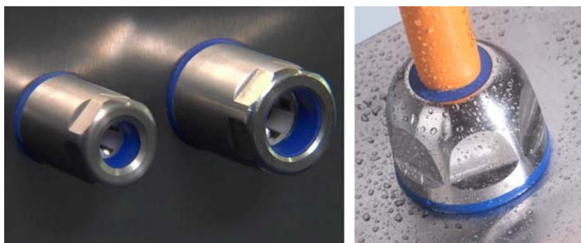
FIGURE 6.67 Hygiene compatible cable glands with seal (blue) directly at the cable entry. The outside of the gland has minimum radii on the hexagon. The connection does not leave an external thread. Due to the presence of a seal with square cross section, the termination between the cap nuts and the enclosure is flush. Photo left: courtesy of Rittal GmbH & Co. KG; photo right: courtesy of Pflitsch GmbH & Co. KG.
