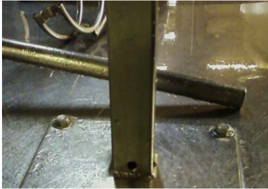
FIGURE 6.37 The leg end is provided with a drain hole to allow draining of any liquids entering the hollow leg. However, in this design, dirt can get in the leg end and complete draining is not possible. The leg end may provide a niche where microorganisms can grow. Despite the drain hole, at below 0°C temperatures, the leg end can still crack under the impact of ice formed within the leg end. The footplate is also not hygienically fastened to the stainless steel floor plate. Courtesy of Stephanie Olmsted, Safeway Inc., © 2016.
