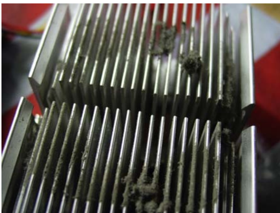
FIGURE 6.61 A cooling device that ventilates the heat produced by electrical equipment to the outside concomitantly accumulates dust and dustborne microorganisms inside the electrical equipment. Moisture- and dust-tight casings with high IP rating will reduce inside buildup of dirt, and therefore are especially recommended in dry material handling areas with high dust loads. Regular cleaning of the interior of electrical devices by vacuum is also a suitable option, but blowing with compressed air even in the presence of a dust extraction system is not recommended (Moerman, 2011).
