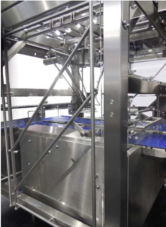
FIGURE 6.57 Clear plastic covers/guard. Frank Moerman, ©2016.
