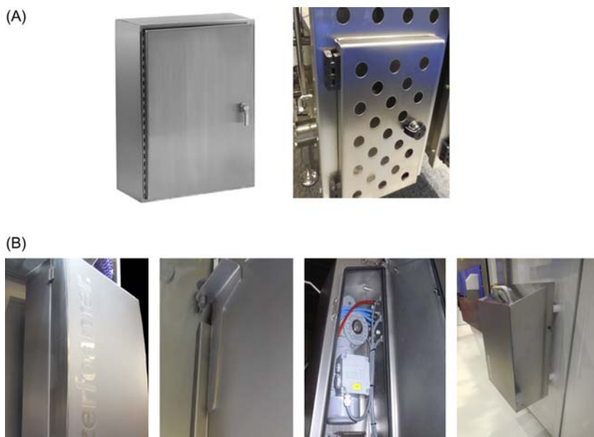
FIGURE 6.55 (A) Continuous and piano hinges are not allowed (Frank Moerman, © 2016). (B) From left to right: block hinges lift-off type, pin hinges with removable pins or concealed hinges should be used. An alternative could be a hingeless cover fixed by means of two small screws at both sides. First and second photo, courtesy of Heinen Freezing GmbH & Co. KG; third photo, courtesy Den Rustfri Stålindustri Kompetencecenter; fourth photo, courtesy IQF Frost AB; Frank Moerman, ©2016.
