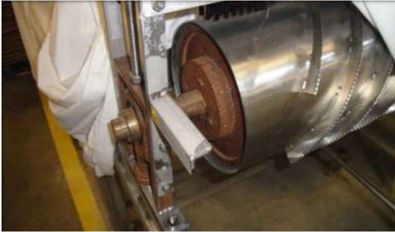
FIGURE 8.14 Stainless-steel shell and knives of the roller are combined with roller ends in mild steel. As mild steel is less noble than stainless steel, it will corrode. Work in black steel and stainless steel must always be kept separate. Courtesy of organization Sanitary Design Workshop, © 2016.
