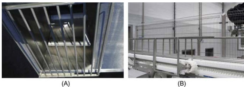
FIGURE 6.58 (A) Bars made of full stock rod preferably with small cross section and positioned in a vertical direction (easily cleanable from all directions). (B) If weld mesh guards are used, they should have a minimum number of horizontally running wires. Courtesy of NTF-Aalborg A/S.
