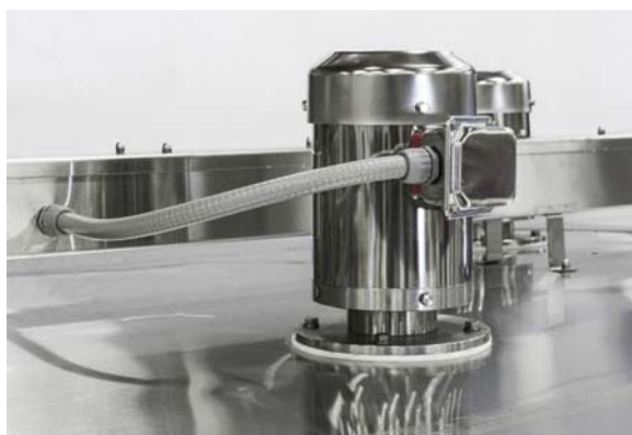
FIGURE 6.54 Wash-down motor. However, it is preferable to avoid hosing of motors, outlets, and electrical cables. The electrical connection to the motor should be waterproof and the cable gland of the motor should be positioned in a direction pointing away from the food contact zone and away from direct spraying when cleaning. Courtesy of CES NV.
