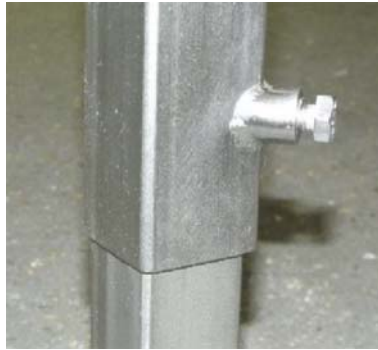
FIGURE 6.4 Penetration of hollow sections of equipment such as frames with bolts is not allowed. Hollow sections shall be hermetically sealed (Kold et al., 2016).
