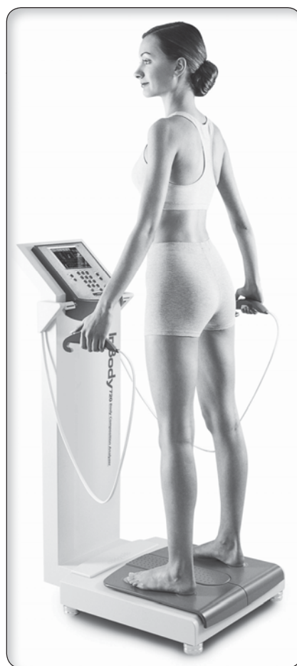
Figure 12.5 An eight-mode bioelectrical impedance device.
