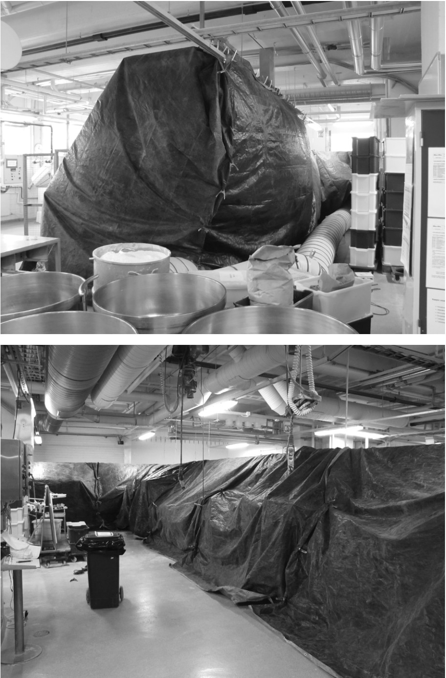
Figure 4.3 Insulation of food processing equipment prior to heat treatment. (Photograph courtesy of Lara Schaumann)
